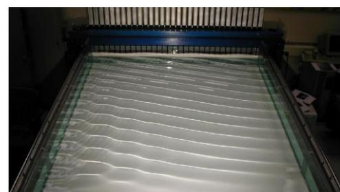
**DIRECTIONAL WAVES IN A COMMERCIAL TEST TANK**
